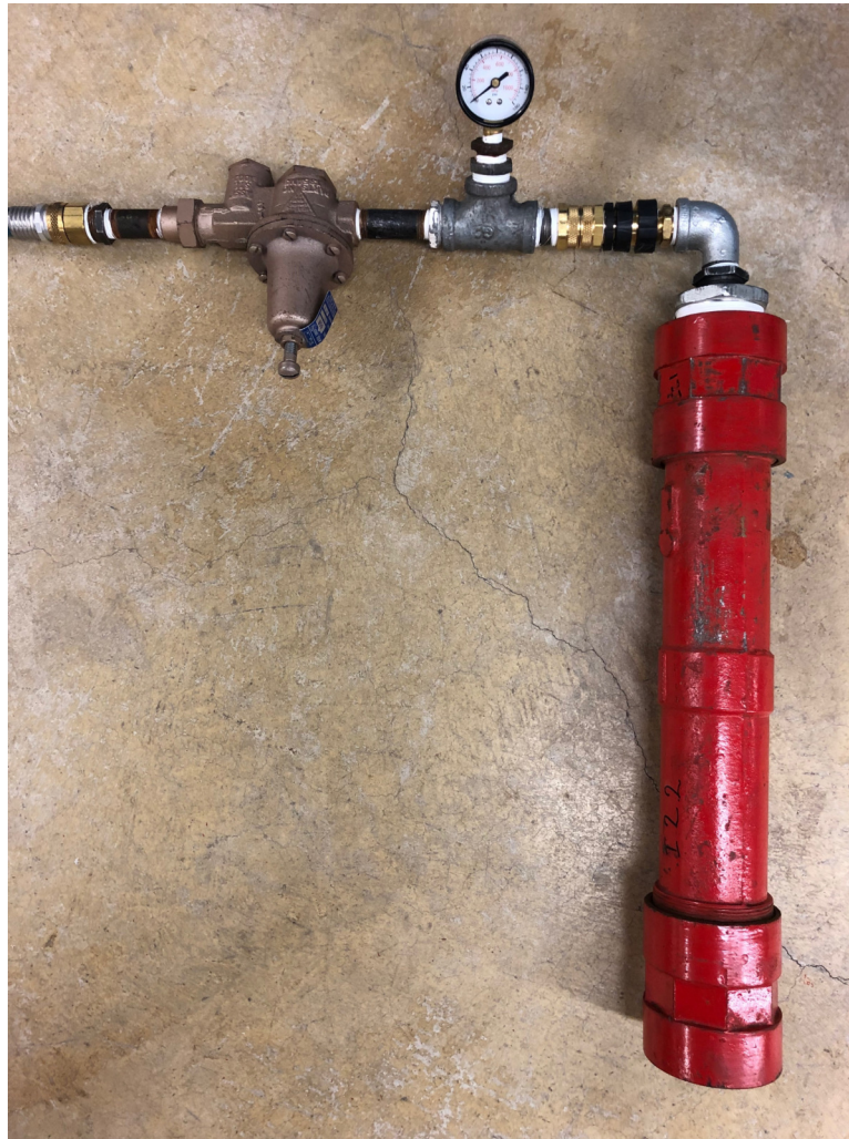
Figure 4.10: Test setup for determining cup seal leak rate
