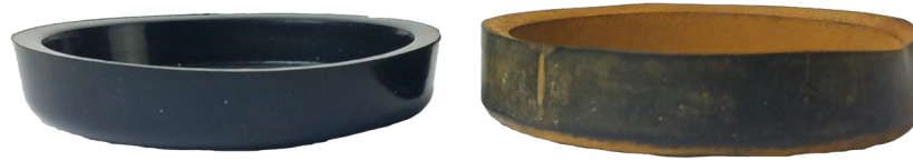
Figure 4.8: New cup seal (left) and a used cup seal (right) for the India Mark II/III hand pump system
