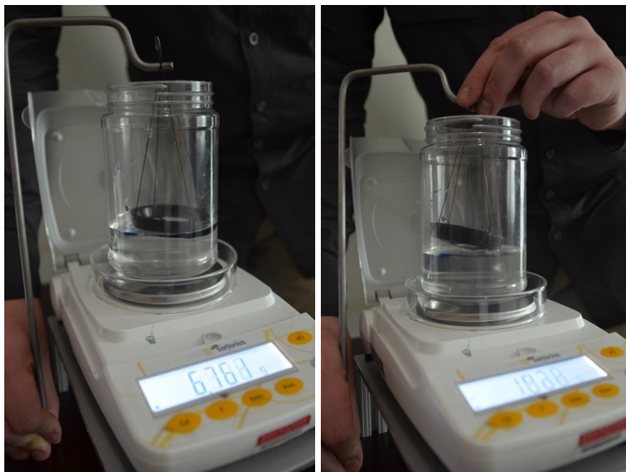
Figure A2.1. Setup of seal volume test.
