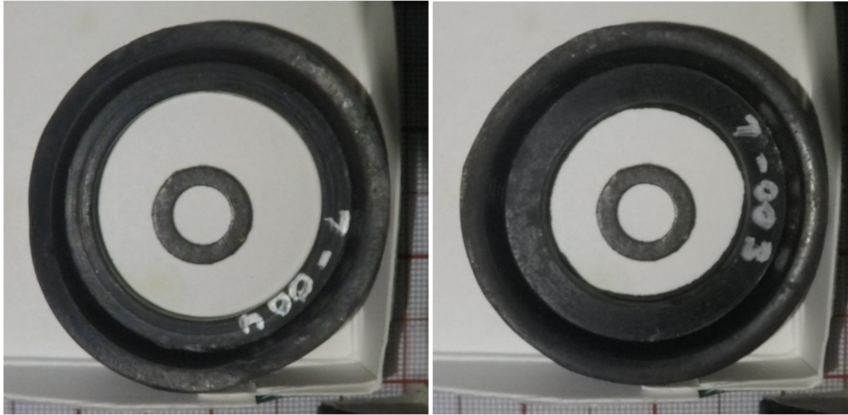
Figure A2.2. Differences for the inner diameter – seals purchased at store 7.
