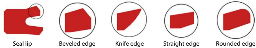
Figure 5.10: Different lip geometries [13]
